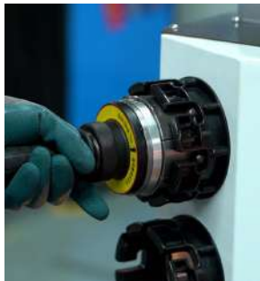
Quick-change system for easy replacement of dies
