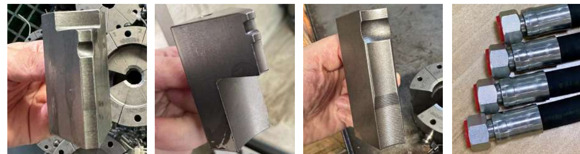
Crimper Dies Type One Bubble Crimping Dies
