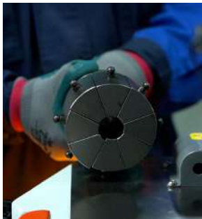
12 sets of dies are prepared for most of crimping ranges.
