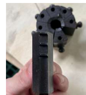
Crimper Dies Type Two Bubble Crimping Dies
